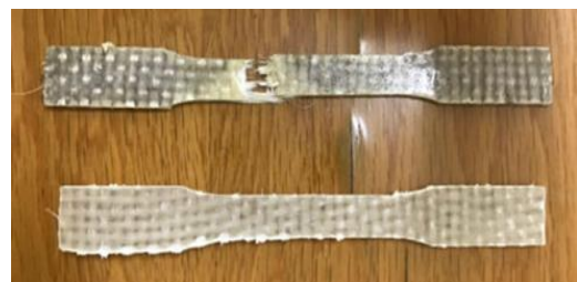
Figure 4. Tensile Test Specimens (Woven)
