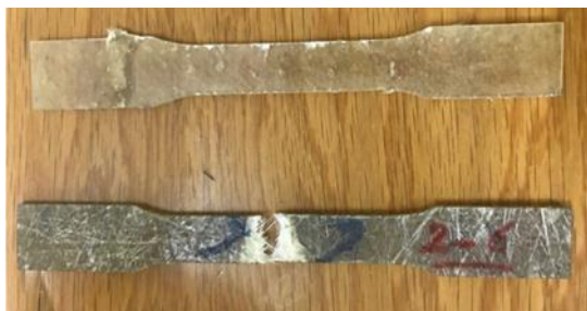
Figure 5. Tensile Test Specimens (Random)
