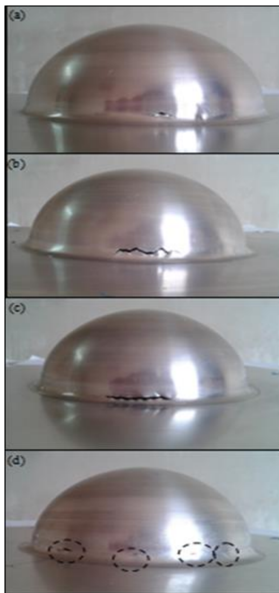
Figure 4. Failure modes in TPIF process
