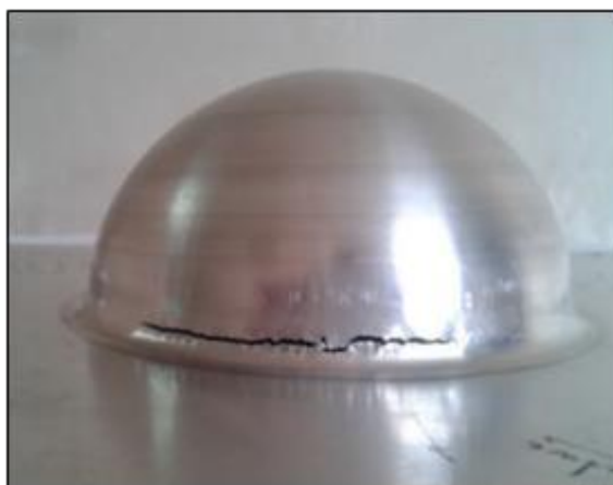
Figure 5. Failure modes in TPIF process with rapid crack
