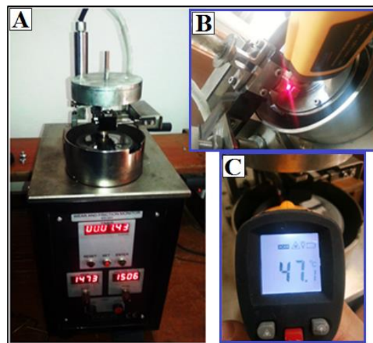
Figure 1. A: Pin-on-disc tribometer, type (Ed-201 wear and Friction, monitor), B: Measuring of contact temperature, C: Example for a measured temperature value.
