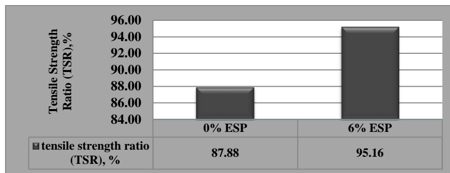
Figure 8. Effect of Egg Shell Powder (ESP) On Tensile Strength Ratio of Asphalt Mixtures.
