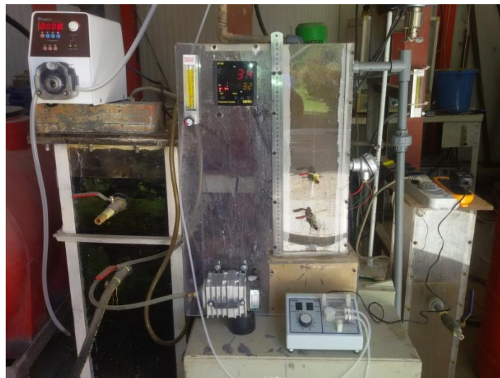
Figure 2. Photograph of the pilot-plant system.
