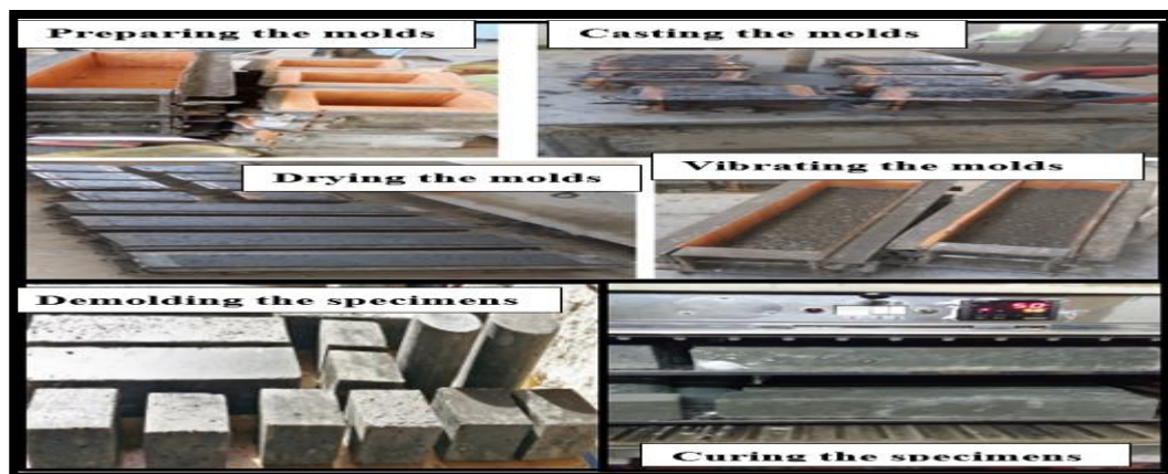
Figure 3. Preparing the geopolymer lightweight concrete samples
