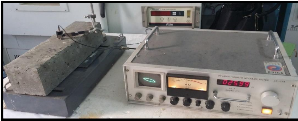
Figure 4. Resonance frequency method
