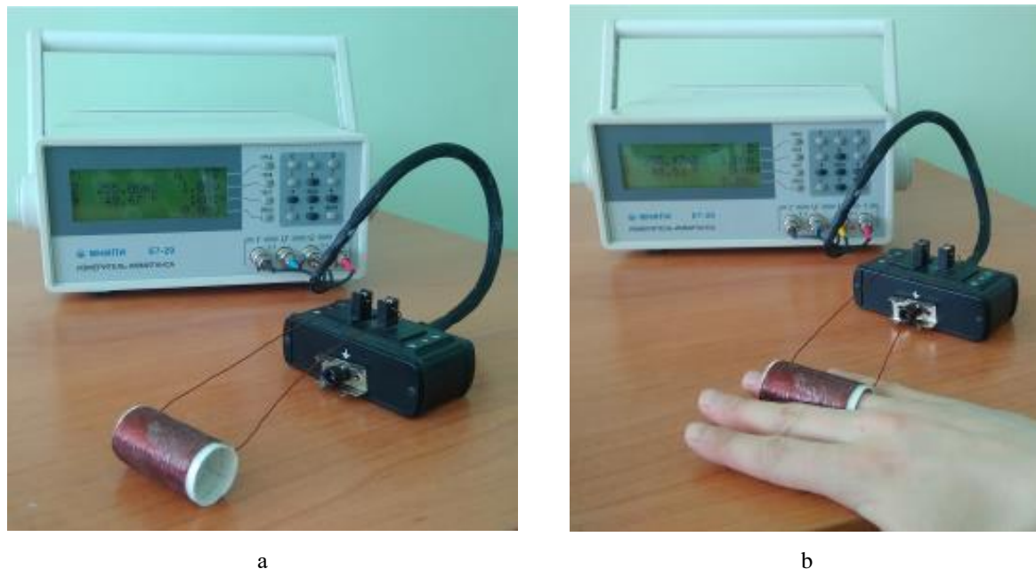
Figure 1. Measuring coil: in calibration mode (a) and in measurement mode (b).
