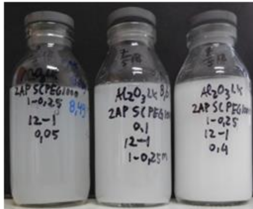
Figure 7. The visual appearance of the nanofluids with the different concentrations of the \text{Al}_2\text{O}_3 nanoparticles after preparation. From left, the first to third bottles are nanofluid with the \text{Al}_2\text{O}_3 concentration of 0.0125 % vol, 0.025 % vol, and 0.1 % vol, respectively.
