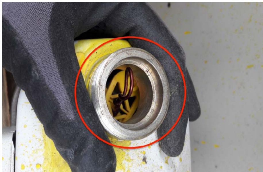
Figure 1. Locking the engagement lever of the recording mechanism
