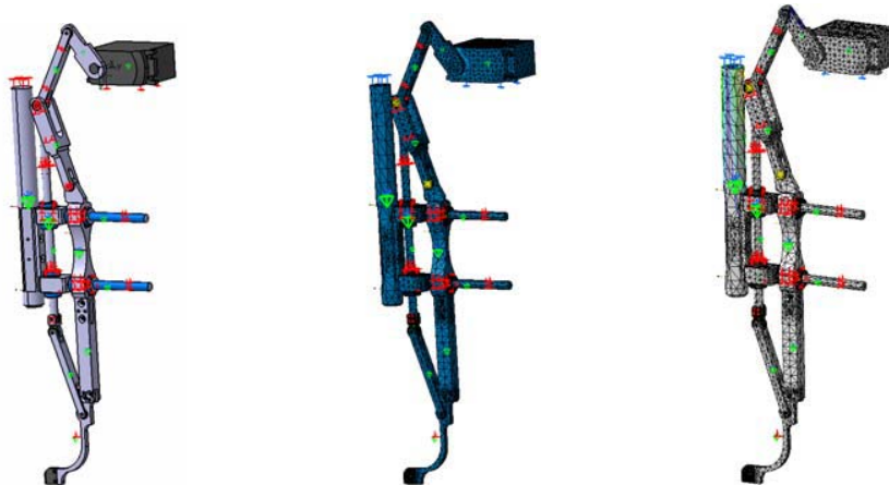
Figure 7. Structural analysis of the prehensor module.
