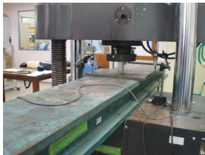
Figure 2. Test setup of stub column.
