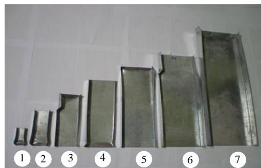
Figure 12. Failure patterns of stub channels.
