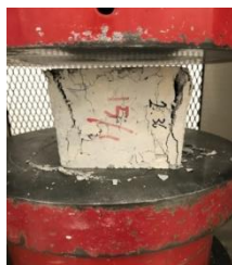
Figure 5. Concrete cube of normal concrete after compression test.
