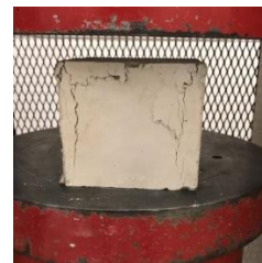
Figure 6. Concrete cube of kenaf fibre composite after compression test.
