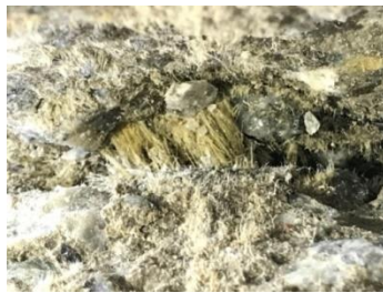
Figure 7. Kenaf fibre inside concrete cylinder specimen.
