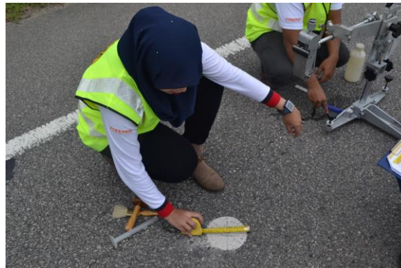
Figure 4. Measuring texture depth using the Sand Patch Method.
