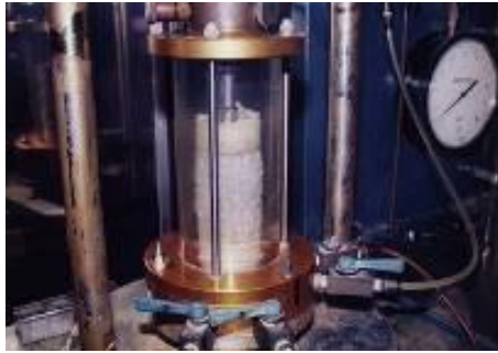
Plate 3. Test situation of Tri-axial test
