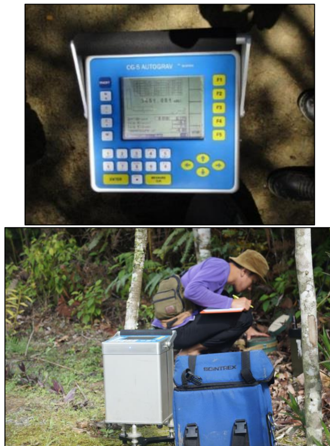
Figure 4. Data acquisition at site using gravitometer
