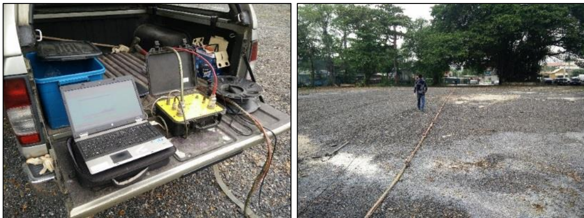
Figure 1. Data acquisition at site using MASW technique
