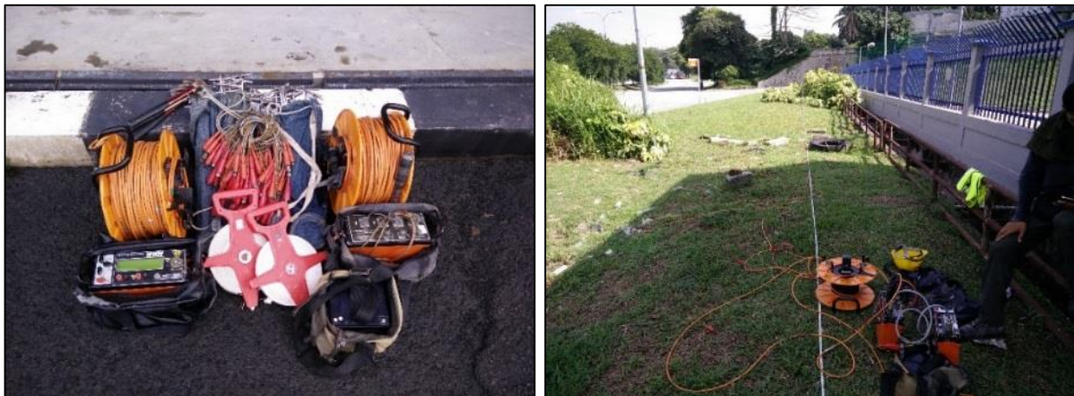
Figure 2. Data acquisition at site using Resistivity technique
