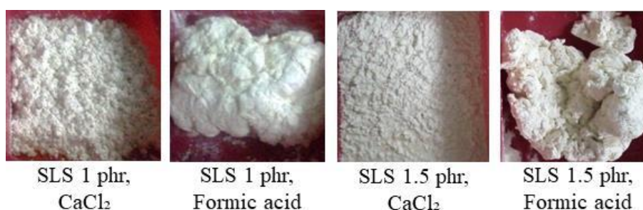
Figure 4. Wet coagulum of hydrogenated natural rubber stabilized with SLS.
