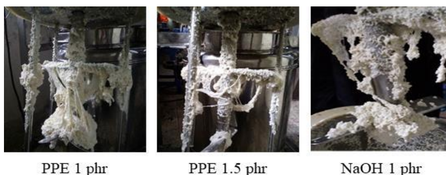
Figure 2. Instability of natural rubber colloidal system during hydrogenation.
