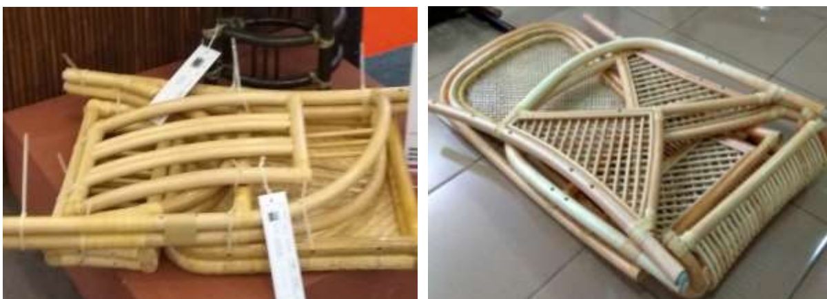
Figure 4. The final result of the knock down rattan furniture construction system for the global market
