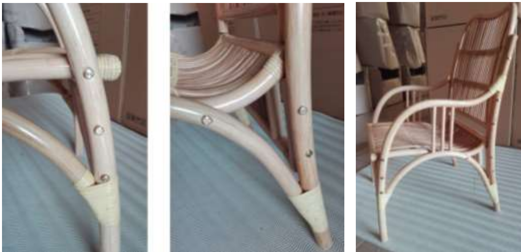
Figure 3. Application of nuts connector on bolts joint connector (JCB) in rattan chairs.
