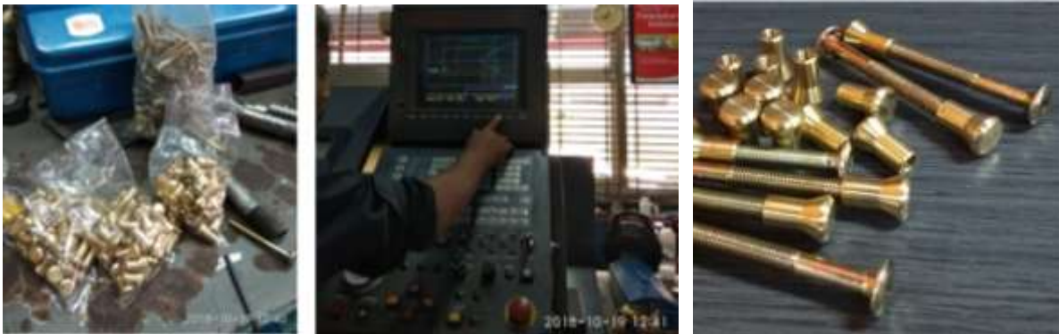
Figure 2. Manufacturing process of nuts connector product on bolts joint connector (JCB) for knock down systems on rattan furniture.
