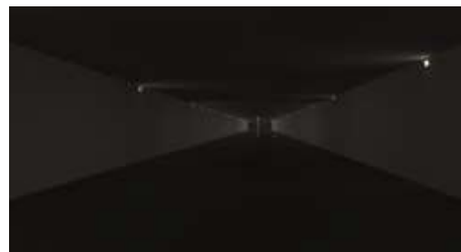
Figure 7 Simulation of tunnel lighting at exit zone
