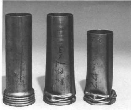
Fig. 3. Axisymmetric and nonaxisymmetric crush mode (Jones, 1989)
