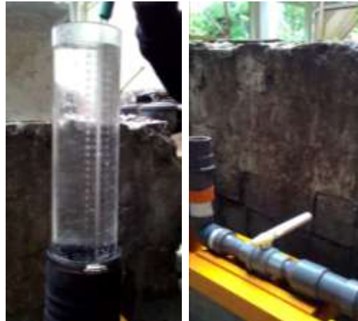
Figure 2. Permeability test with Falling Head Permeability
