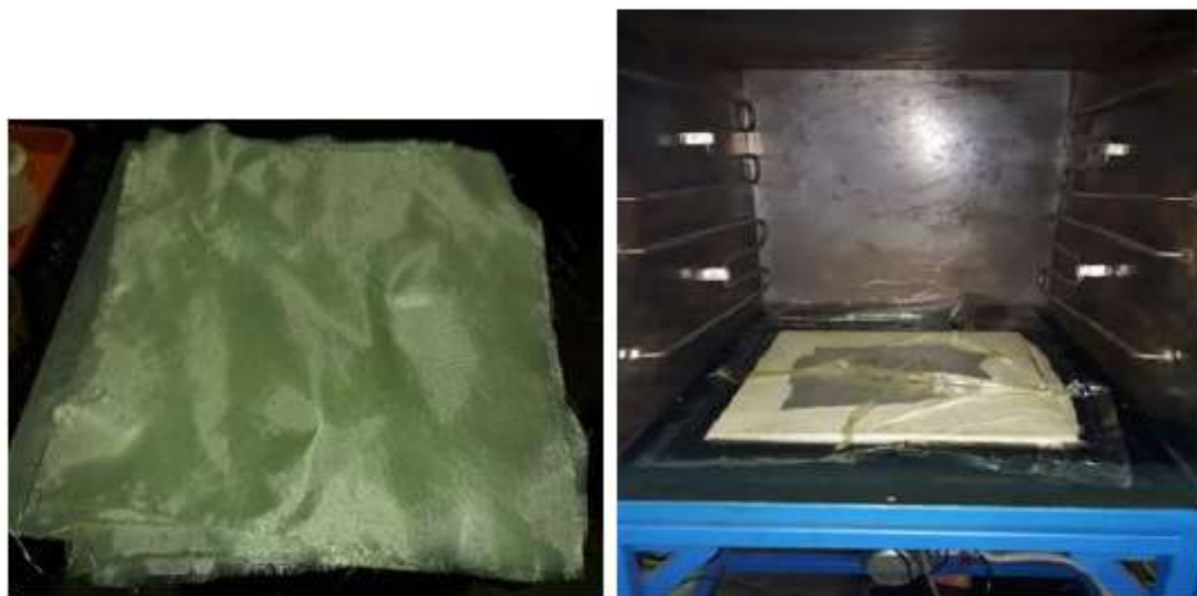
Figure 1. Woven glass fiber (left) and wrapped specimen in the oven (right)
