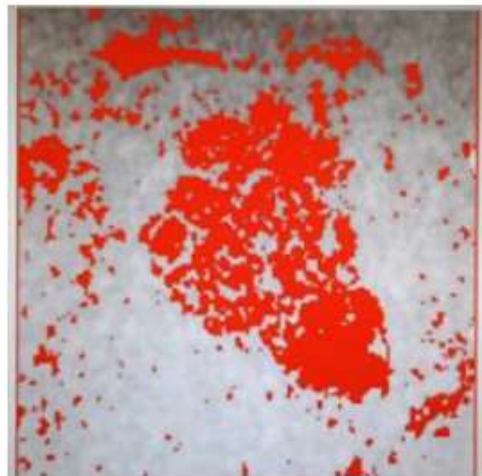
Figure 5. TTU result of the specimen after the blast loading
