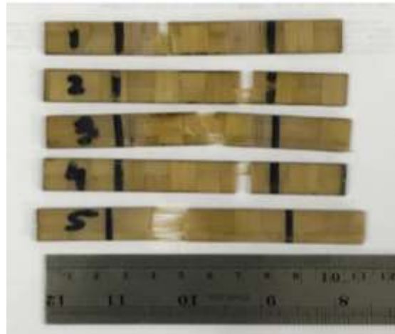
Figure 5. Tensile test results specimen
