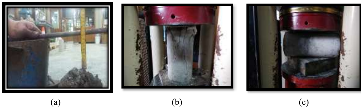
Figure 2. Testing of a slump (a), compressive strength (b) and tensile strength (c).
