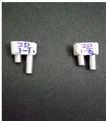
Figure 11. LM25 is low in ductile property.
