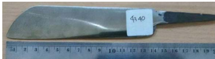
Figure 2 Steel knife 4340 manual forging results
