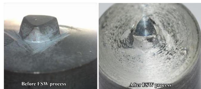
Figure 9. Physical appearance of tool wear for triangle tool
