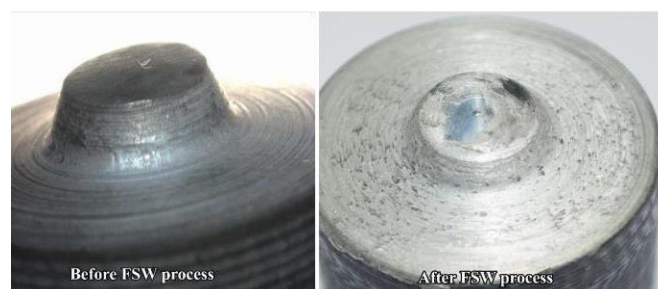
Figure 10. Physical appearance of tool wear for tapered tool
