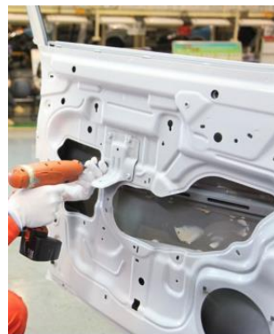
Figure 1. Electric wrench fastening sheet metal parts.
