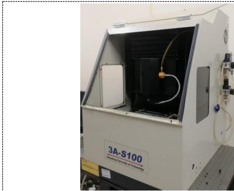
Figure 1. Micromilling machine tool 3A-S100.
