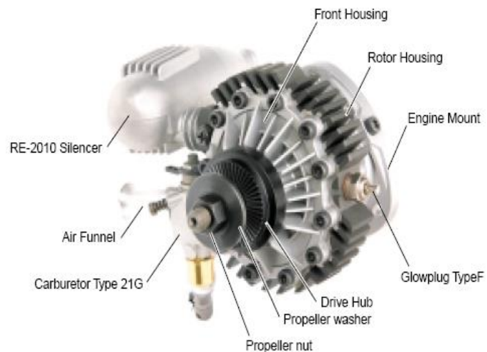
Figure 2. Basic engine parts.
