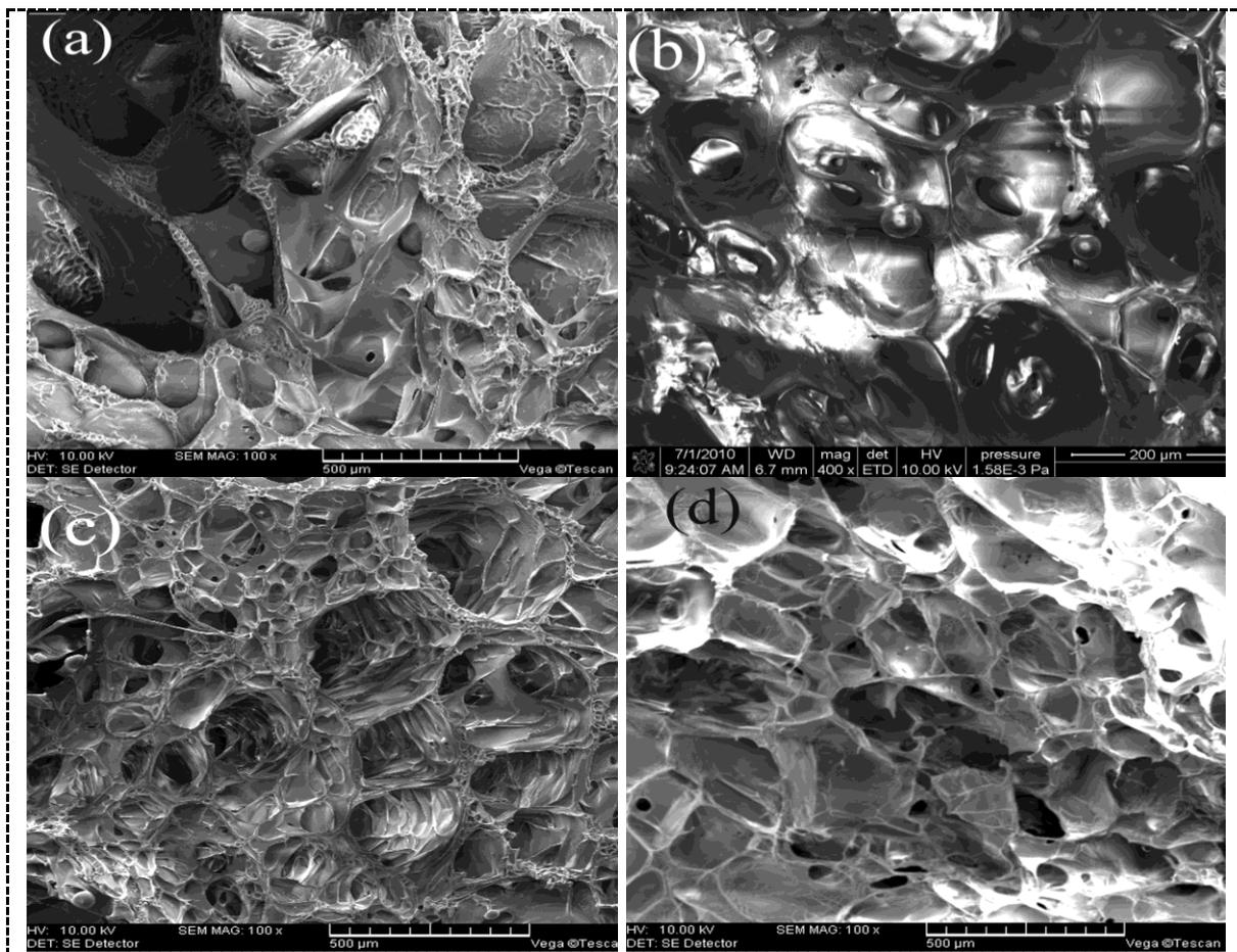
**Figure 1.** SEM images of PLGA microspheres /P(NIPAAm- co-AAm) hydrogel combination systems:(a), (b), (c) microsphere-loaded hydrogel combination systems; (d) porous P(NIPAAm-co-AAm) hydrogel.
