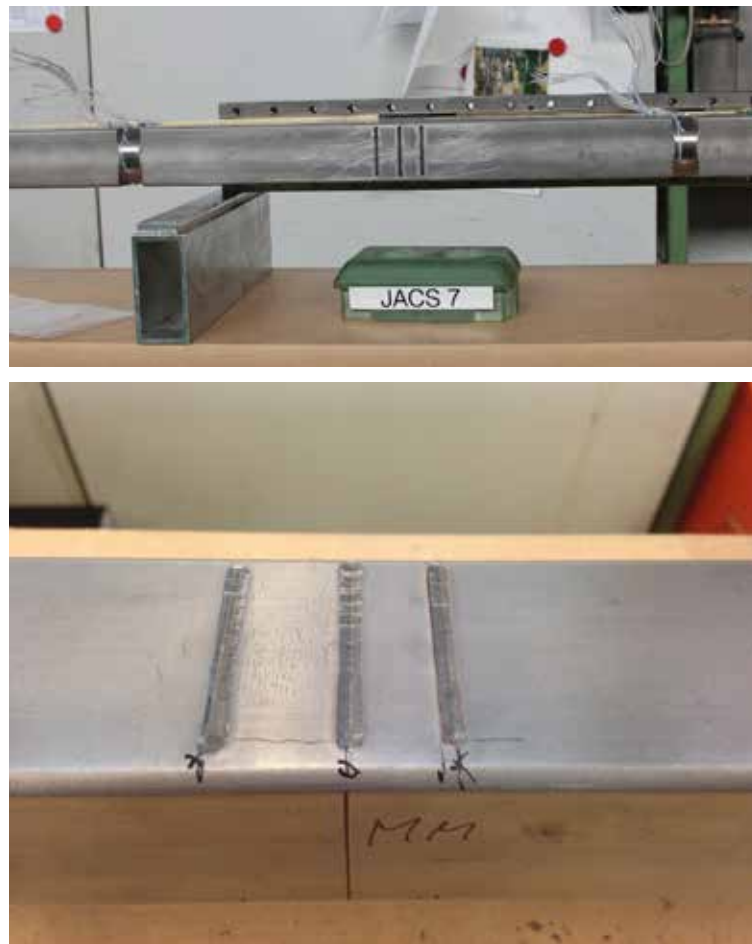
Figure 4. A general view (top) and a closeup view (bottom) of the UP-treated conductor CSJA7.
