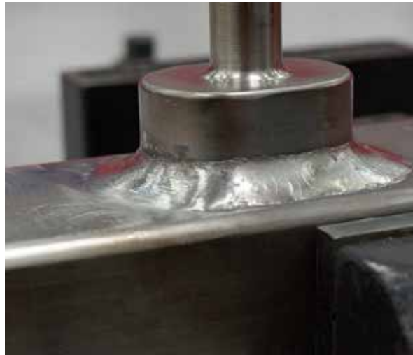
Figure 1. Helium inlet after welding.
