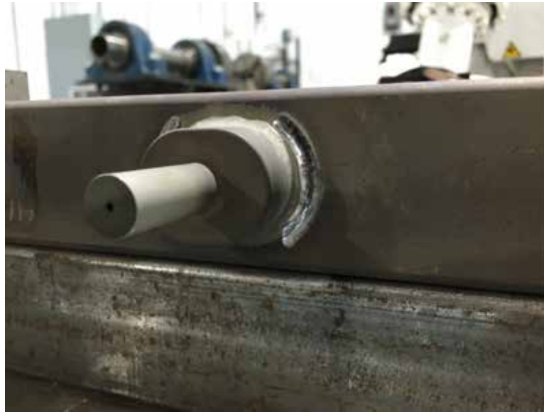
Figure 3. An inlet treated with ultrasonic peening.
