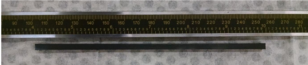
Figure 1. Square cross section ETP core
