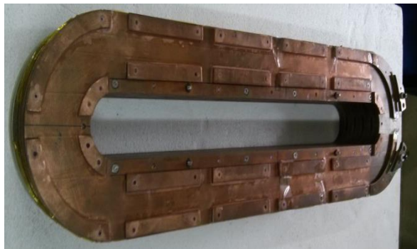
Figure 8. Developed HTS pole coil
