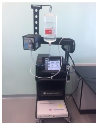
Figure 1. Microwave ablation system (at Center of Scientific Equipment for Advanced Research, Thammasat University).
