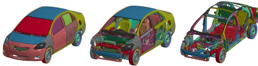
Figure 5. The detail FE model of Toyota Yaris passenger sedan 2010.
