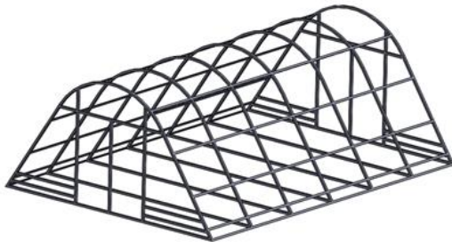
Figure 1. The parabola greenhouse solar dryer model
