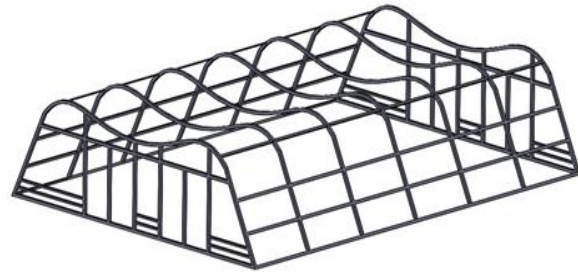
Figure 2. The sinusoidal greenhouse solar dryer model
