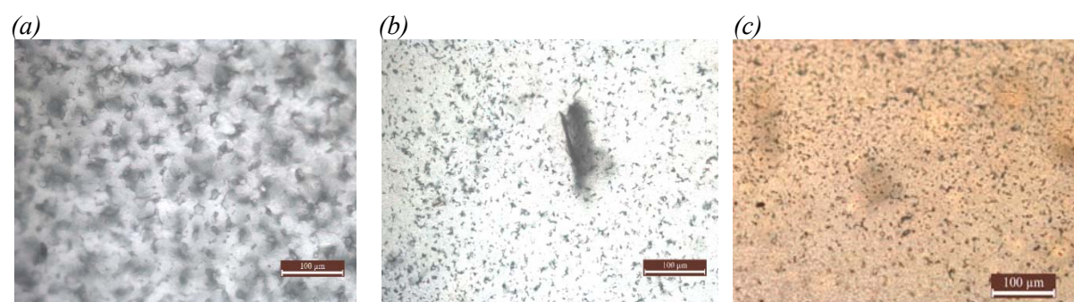
Figure 4. Images obtained by polarized light microscopy for films based on native PCL (a) and PCL filled with NCC (b) and NCC-PLLA (c).
