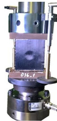
Figure 3. Edgewise compression test setup.
