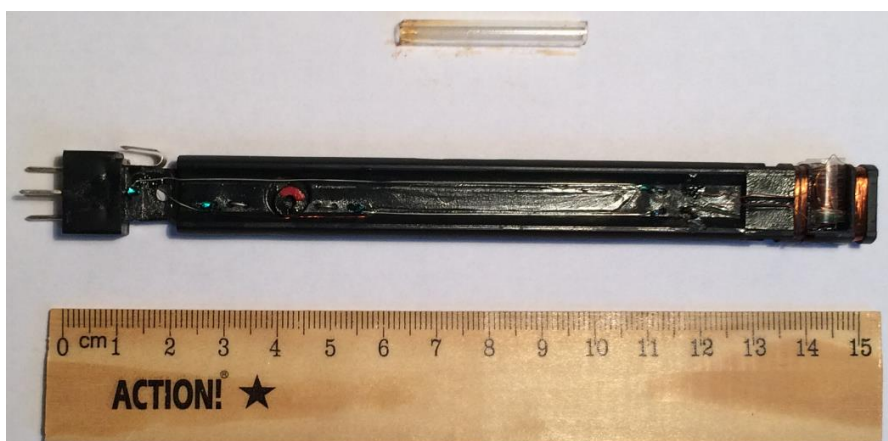
Figure 2. Measuring probe and container for the studied medium.
