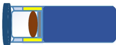
Figure 1. Schematic of the position of the template inside a modified tube.
