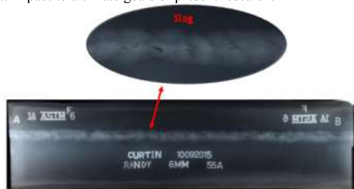
Figure 3: Radiographic Film for 55A Weld Sample
