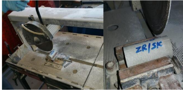
Figure 4. Mechanical saw applied to flatten ends of samples.
