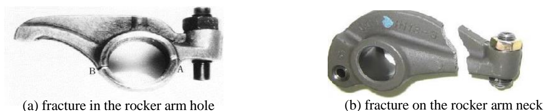
Figure 1. Rocker arm fracture position [3]
