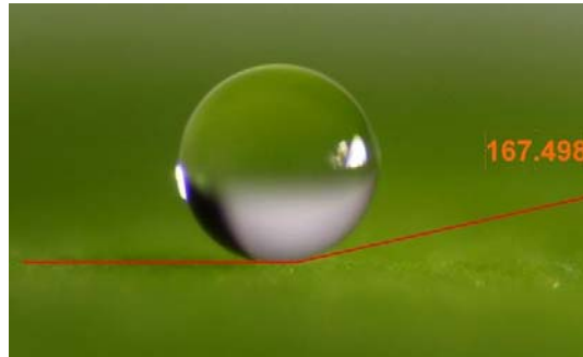
Figure 7. The contact angle between the water droplets with taro leaf surface
