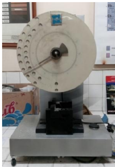
Figure 7. Charpy impact testing machine
