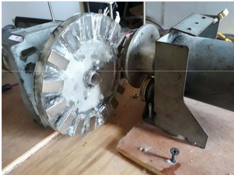
Figure 5. Prototype of magnetic gear axial mounted on test bench ( d = 0.5 \text{ mm} )
