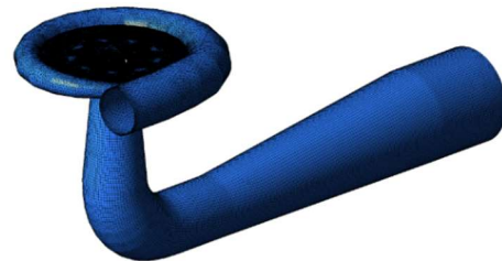
Fig. 3 Flow path of the pump turbine
