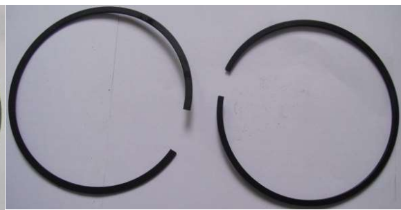
Fig 2. Piston ring after QPQ treatment
