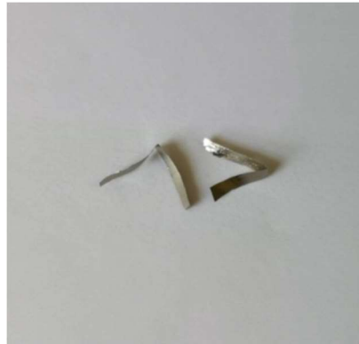
Figure 4. The picture of \text{Au}_{40}\text{Cu}_{30}\text{Pd}_{10}\text{Si}_{20} alloy ribbons after bending deformation through 180^\circ
