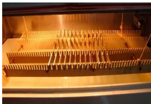
Figure 2. Accelerated corrosion test state of specimens
